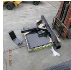
Fig 2 Propping system pre assembly.
